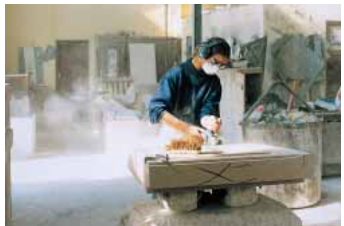
Workplace inspection aids understanding of the job demands and risks. This stonemason is exposed to hand transmitted vibration, noise, and silicaceous dust
