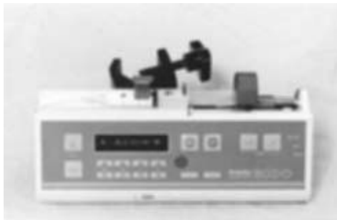
Figure 11.3 Syringe pump for milk.
